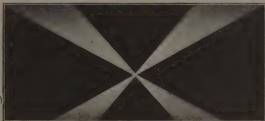
FIG. 57. Photograph of rays of light leaving a hemispherical condenser. The bases of the two lower cones are at the top surface of the condenser; their meeting-point is the position of the specimen; the two upper cones represent the rays which have passed through the fluid part of the specimen.
